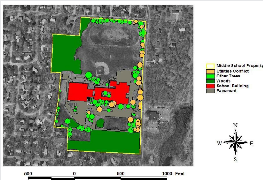
FIGURE 8.5 Trees conflicting with utility lines.
