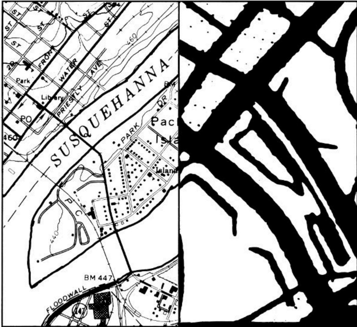
Figure 3.4. Area near Northumberland, Pennsylvania, as portrayed on topographic maps at 1:24,000 (left) and at 1:250,000 enlarged to roughly 1:24,000 for comparison (right).
